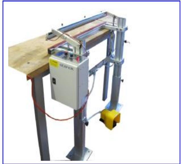
*These pneumatic sealing device is suitable for rapid and simple sealing of film widths up to length of 1000 mm.*
