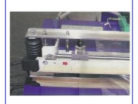
Sealing lenght (mm) 600 Sealing width (mm) 4 Bar opening (mm) 20 Film thickness (mm) 2x0,40 Connection 230V/50-60 Hz Degrees protection IP 20 Vacuum pump Q=6m3/h dryWeight Kg. 69 900x220x330h Dimension (mm))
